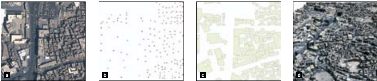
Figure 2: The figure shows a 250 x 250 m large area collected over Sana'a and the derived exposure products (a), point assessments (b), building footprint map (c) and building volume map (d)
